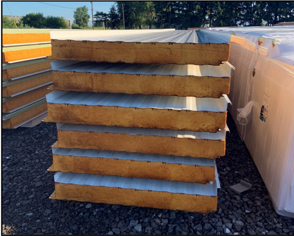
Insulated Metal Panel cross-section. 6" of solid foam insulation sandwiched between 2 pieces of steel cladding.
