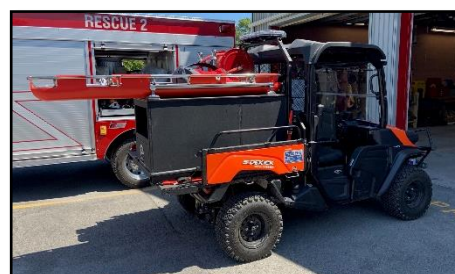
Rescue Stretcher (Stokes Basket) Mounted on the UTV Fire/EMS Skid-Unit
